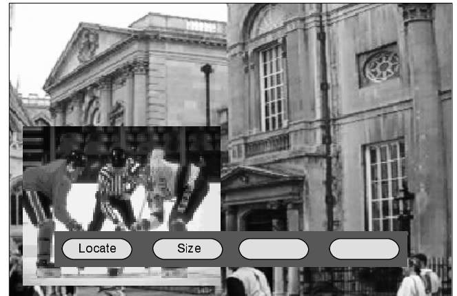
Pressing the PIP button a second time when viewing a widescreen picture will cause the Locate and Size reminder to be displayed. Simply choose the coloured button of the remote control if you wish to move or size the picture.
